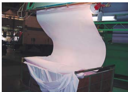
▲ top left: shirts/school uniform bottom: drying the textile after dipping into Photocatalyst solution
