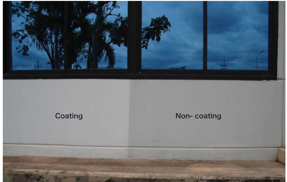
▲ Outdoor optical coating paint test. After 45 days (outside factory wall of a Japanese company / Thailand)
