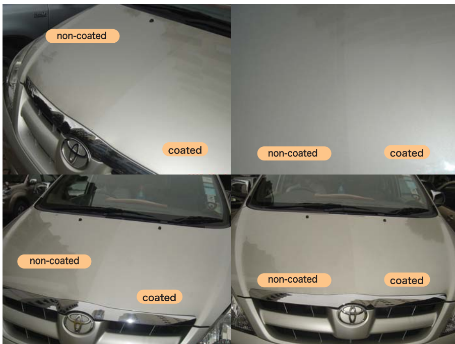
▲ Experimenting self cleaning on a passenger car that was coated with the titanium dioxide photocatalyst paint on the body. Can clearly see the difference between the coated surface and non-coated surface. With silica's high water friendliness, it makes it easy to get the dirt off in the rain.
