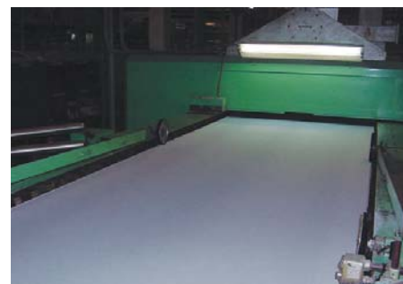
▲ top left: shirts/school uniform bottom: drying the textile after dipping into Photocatalyst solution
